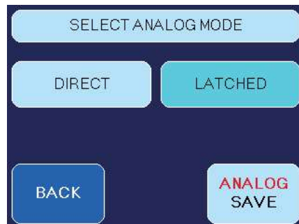
Fig. 7 Select Analog Mode - Latched
