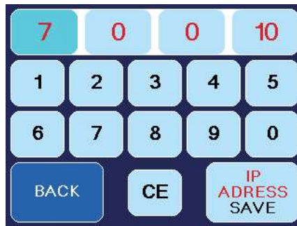
Fig. 17 Screen to adjust the IP-address and Subnet mask
